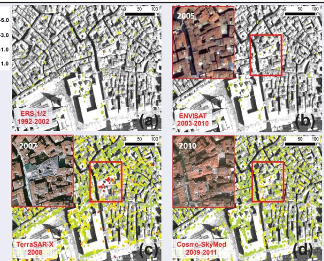
Fig. 6 – Example of temporary high sinking rate due to restoration work of single palaces
