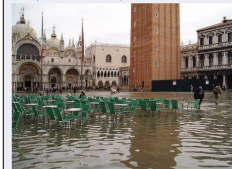
The RSLR, i.e. subsidence plus eustasy, calculated for the last century is about 25 cm. This produced a significant increase in frequency of the "acqua alta" events (Fig. 1).
