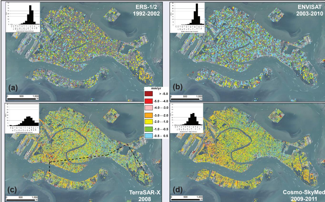
Fig. 3 - Mean displacement rates (mm/year) obtained by IPTA. The histograms represent the displacement frequency distribution computed for the whole city.
