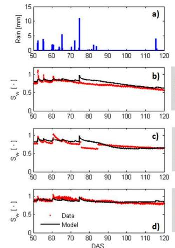
**Fig. 4** Observed (red circles) and modeled (black lines) soil moisture at the monitoring station A, B and C at the depth of 10 cm.
