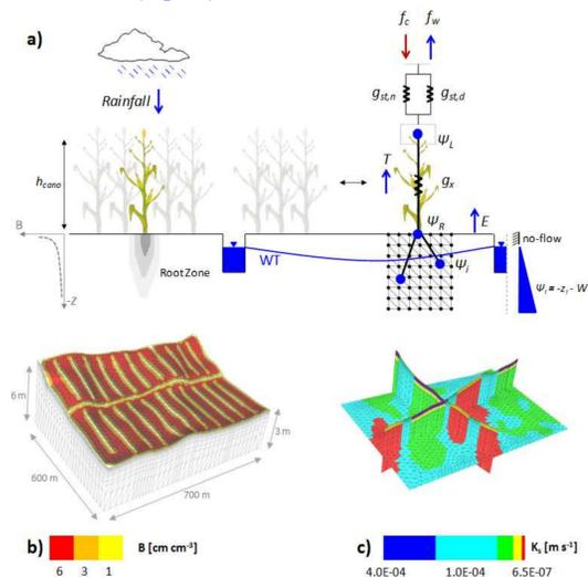
**Fig. 3** Field scale simulations: a) conceptual model, b) simulation grid G2 and root length density  $B$  and c) spatial distribution of saturated hydraulic conductivity  $K_s$ .
