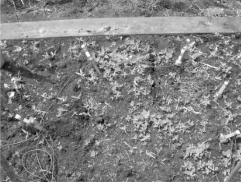
Fig. 8 – Tensiometer location within a test site.
