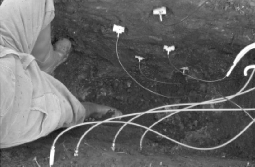
Fig. 9 – TDR probes (upper) and temperature sensors (lower) soon after their establishment.
