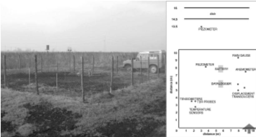
Fig. 7 – A principal test site established in the Zennare Basin with a schematic illustration of the instrument distribution.
